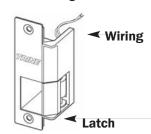
Figure 3. Position of Electric Strike for Right Handed Door.
