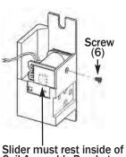
Figure 9. **Coil Assembly Bracket**
