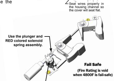
You should NOT see the "X" on top of the actuator cam.
